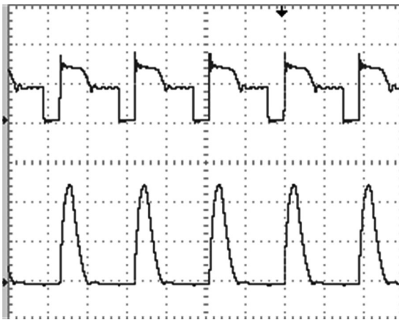
Fig. 14. Drain–source voltage of the switch (upper signal) and output current of T_1 (lower signal), P = 100 W, V_{in} = 230 V_{rms} , V_o = 48 V, V_{DS} = 250 V/div, I = 2 A/div, t = 5 \mu s/div .
