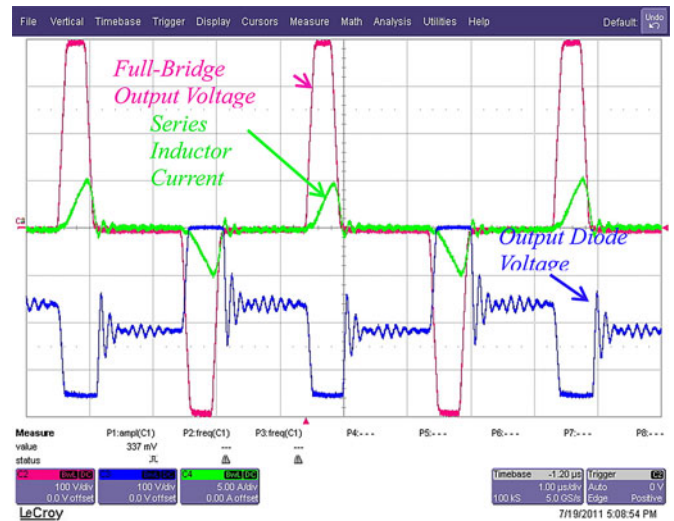
Fig. 16. Proposed converter waveforms at 10% load.
