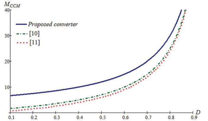
Fig. 8. Voltage gain as a function of the duty ratio of the proposed converter. [10] and [11] under CCM operation and  $n = 5$ .
