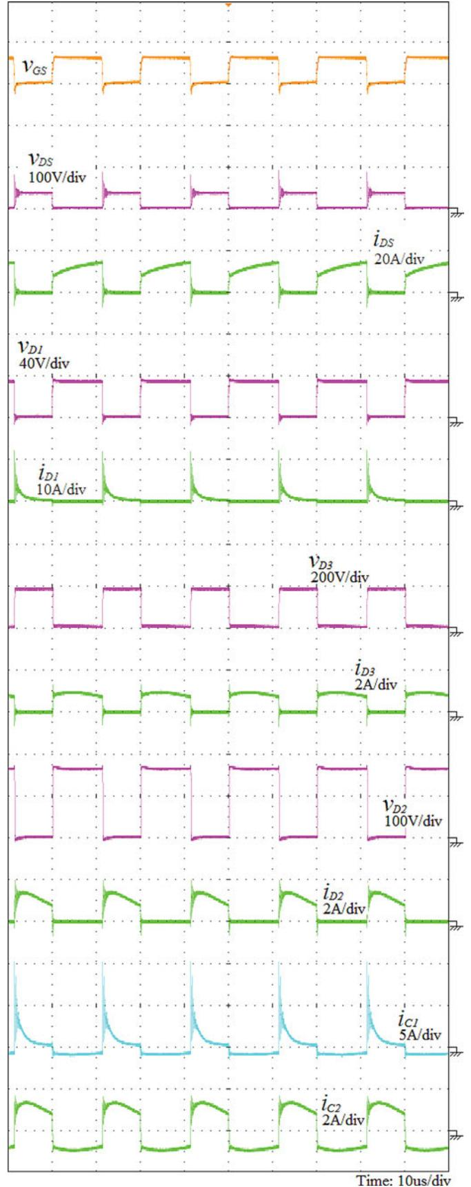
Fig. 11. Experimental waveforms measured by the condition of  $f_S = 50$  kHz,  $V_{in} = 15$  V, and output 100 W.
