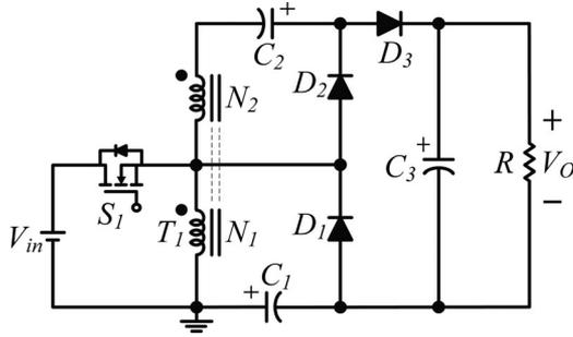
Fig. 2. Circuit configuration of proposed converter.
