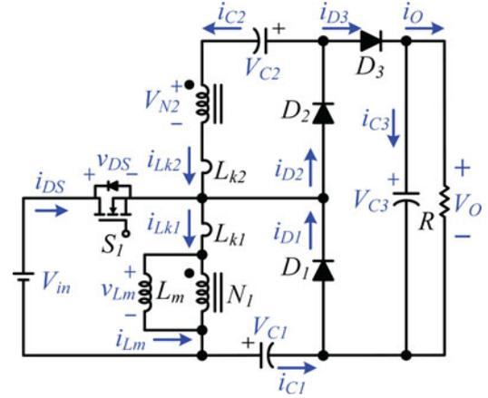
Fig. 3. Polarity definitions of voltage and current in proposed converter.
