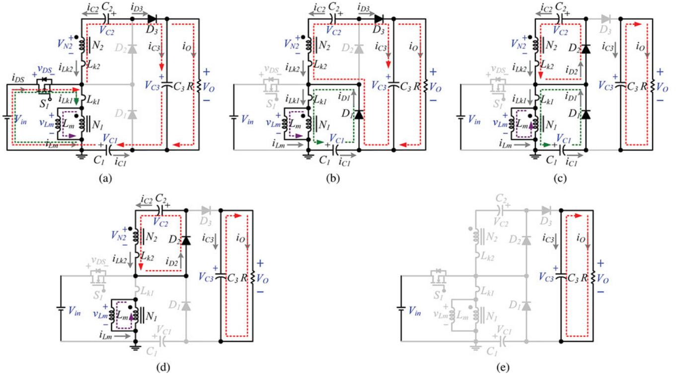
Fig. 7. Current flow path of five operating modes during one switching period at DCM operation. (a) Mode I:  $t_0 \sim t_1$ . (b) Mode II:  $t_1 \sim t_2$ . (c) Mode III:  $t_2 \sim t_3$ . (d) Mode IV:  $t_3 \sim t_4$ . (e) Mode V:  $t_4 \sim t_5$ .
