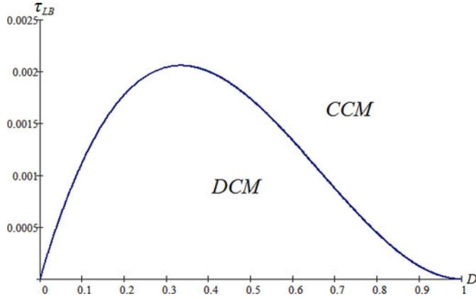
Fig. 10. Boundary condition of  $\tau_{LB}$  of proposed converter under  $n = 5$ .
