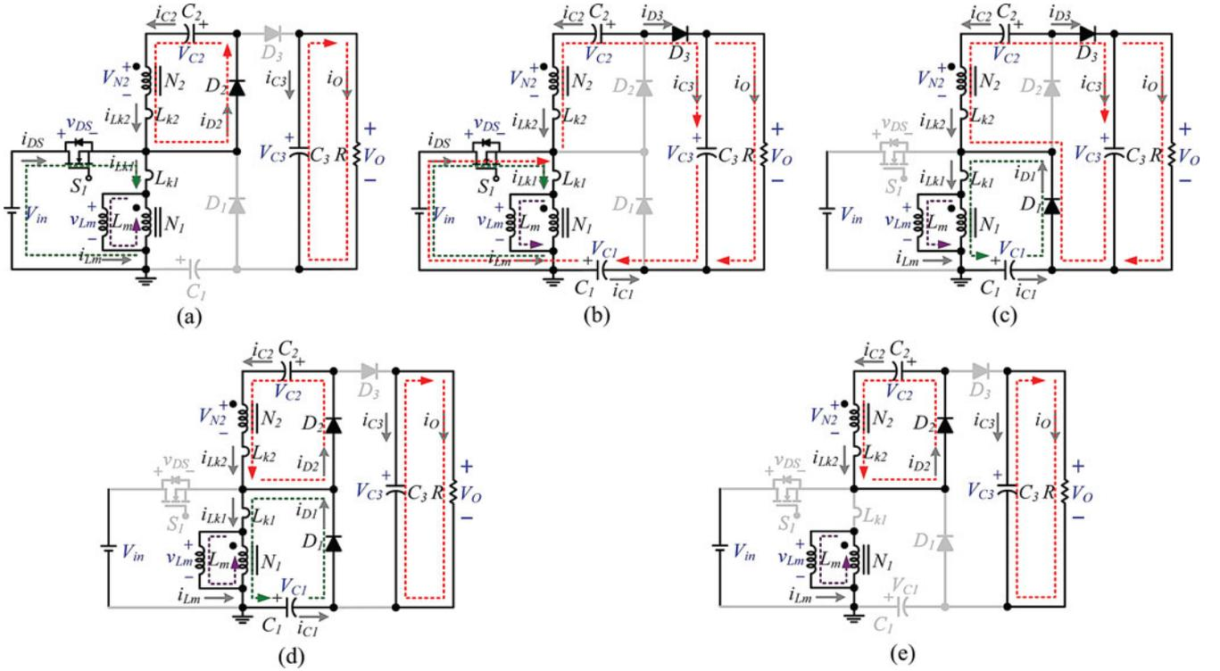
Fig. 5. Current flow path of five operating modes during one switching period at CCM operation. (a) Mode I:  $t_0 \sim t_1$ . (b) Mode II:  $t_1 \sim t_2$ . (c) Mode III:  $t_2 \sim t_3$ . (d) Mode IV:  $t_3 \sim t_4$ . (e) Mode V:  $t_4 \sim t_5$ .
