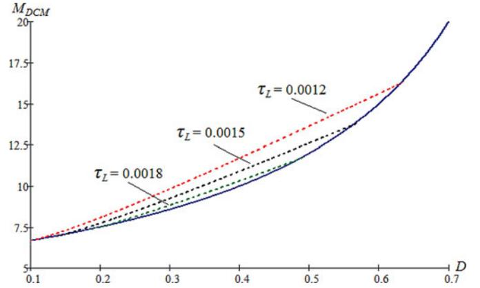
Fig. 9. Voltage gain as a function of the duty ratio of the proposed converter under DCM operation with different  $\tau_L$  by  $n = 5$ .
