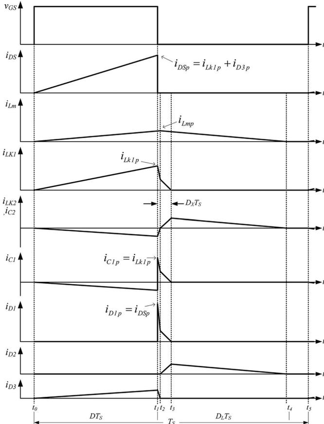
Fig. 6. Some typical waveforms of proposed converters at DCM operation.
