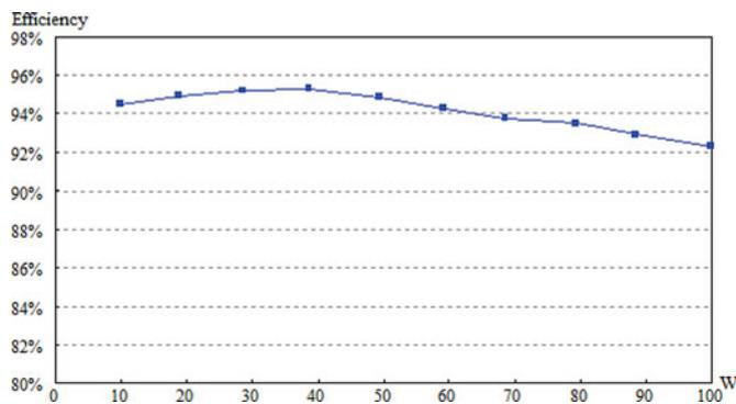
Fig. 12. Measured efficiency of proposed converter.
