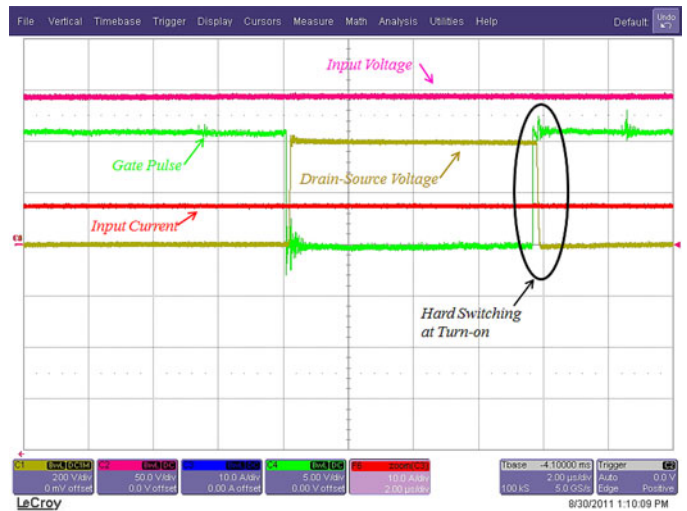
Fig. 22. Conventional interleaved boost PFC waveforms.
