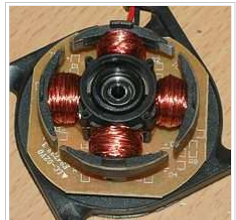
The four poles on the stator of a two-phase BLDC motor. This is part of a computer cooling fan; the rotor has been removed.
