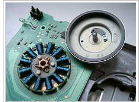
Motor from a 3.5" floppy disk drive. The coils are copper wire coated with green film insulation. The rotor (upper right) has been removed and turned upside-down. The grey ring just inside its cup is a permanent magnet.
