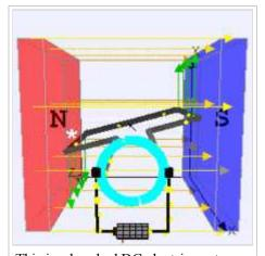
This is a brushed DC electric motor generating torque directly from DC power supplied to the motor by using internal commutation, stationary permanent magnets. Torque is produced by the principle of Lorentz force, which states that any currentcarrying conductor placed within an external magnetic field experiences a force known as Lorentz force. The commutator consists of a split ring 80 degree shows the effects of having a split ring. Other types of DC motors require no commutation.
