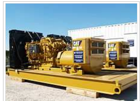
The Caterpillar 3512C Genset is an example of the engine-generator package. This unit produces 1225 kilowatts of electric power.
