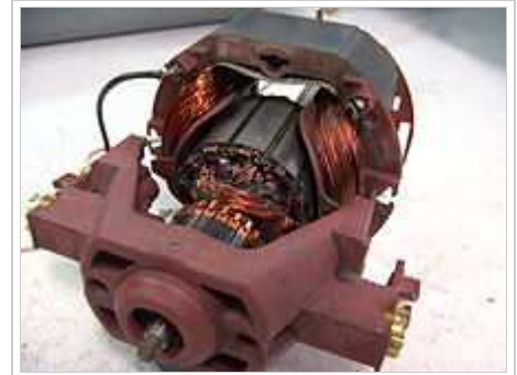
Modern low-cost universal motor, from a vacuum cleaner. Field windings are dark copper colored, toward the back, on both sides. The rotor's laminated core is gray metallic, with dark slots for winding the coils. The commutator (partly hidden) has become dark from use; it's toward the front. The large brown molded-plastic piece in the foreground supports the brush guides and brushes (both sides), as well as the front motor bearing.
