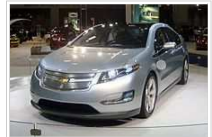
The Chevrolet Volt is a plug-in hybrid able to run in all-electric mode up to 35 miles.
