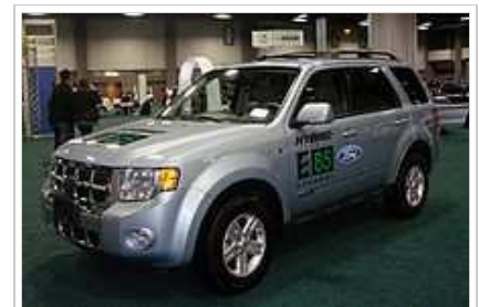
The Ford Escape Hybrid was the first hybrid electric vehicle with a flex-fuel engine capable of running on E85 fuel.
