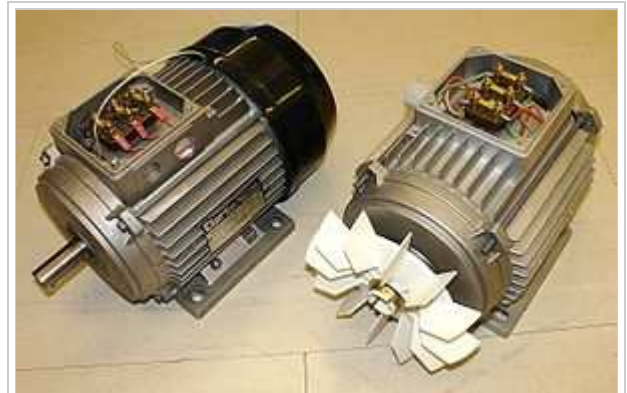
Two three-phase induction motors.
