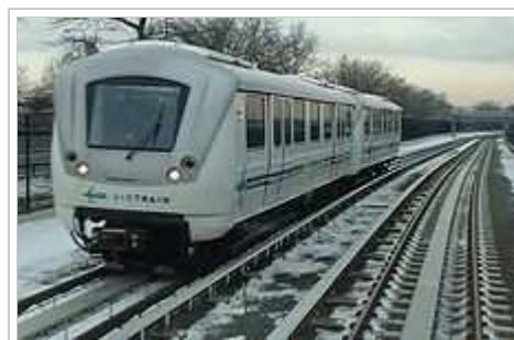
ART trains propel themselves using an aluminium induction strip placed between the rails.
