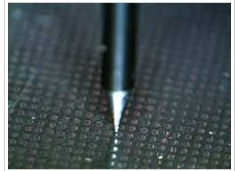
Close-up of the flat passive conductor surface of a motion control linear motor
