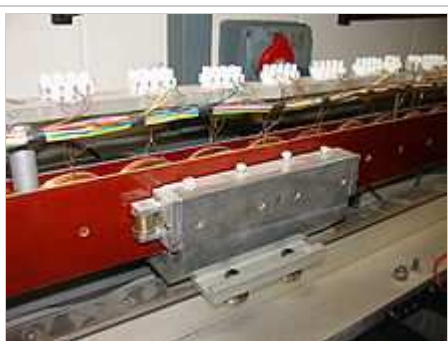
A prototype of linear motor with visible separate coils
