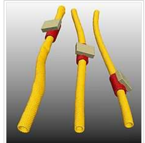
Figure 2.2: Motion of shorter nanotubes (red) along the longer tubes (yellow) from the hotter(top) section of the nanotube to the cooler (bottom) section of the nanotube carrying the metal cargo (gray)
