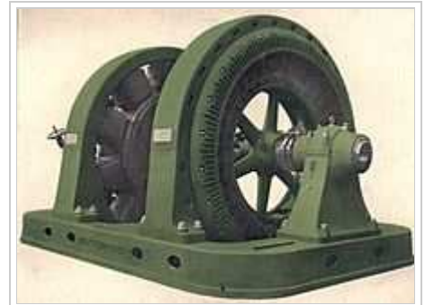
A synchronous motor-generator set for AC to DC conversion.
